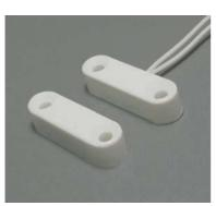
IO 102-16/1 security magnetically contact detector is designed for locking doorways and windows, arranging "trapping" medium as well as locking other elements of buildings with an alarm signal raised to a control panel, concentrator or central surveillance system by opening reed switch contacts.
