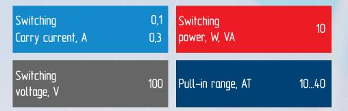
Any DC combination of V&A not to exceed the Switching power.
