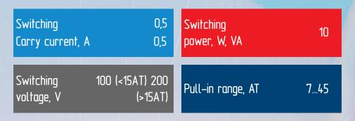
Any DC combination of V&A not to exceed the Switching power.
